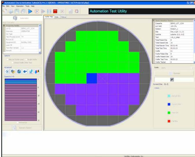
The **Automation** screen provides real-time statistics on lot and wafer yields, overall test progress, and color-coded die binning information. The **Operator Mode** screen shown here limits access to some tools to prevent unauthorized modifications to test plans and reports.
