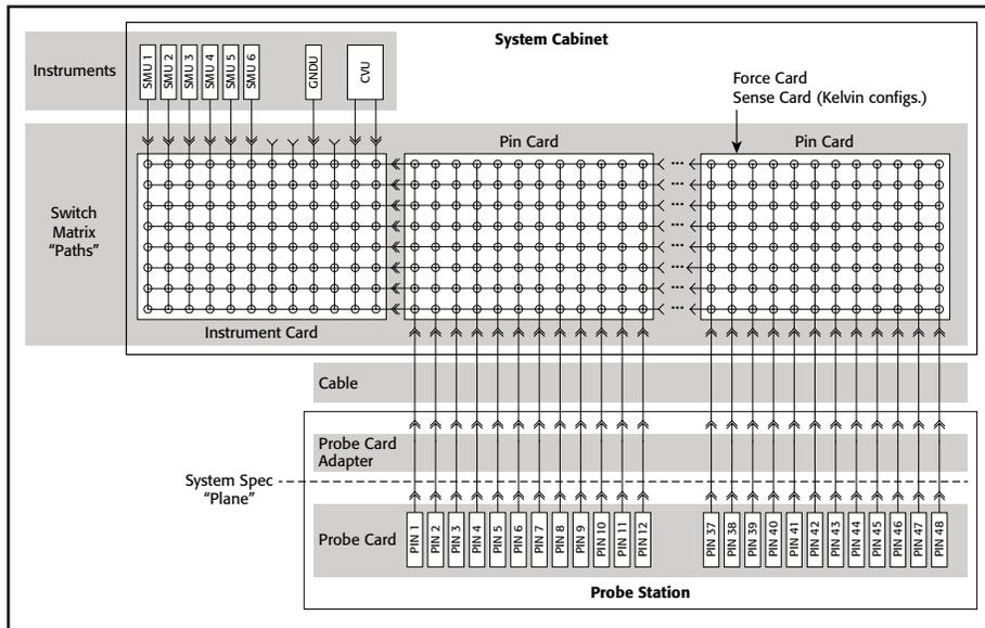
Every S530 system is made up of five layers: instruments, pathways, cable interface, probe card adapter, and probe card.
