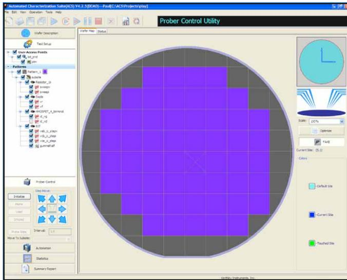
This *Prober Control* screen supports dynamic navigation at both the wafer and cassette levels, as well as interactive test execution. By freeing the engineer from the constraints of the conventional linear test flow, this capability greatly accelerates test plan development by allowing for immediate verification of the test results; it also speeds lot disposition by allowing engineers to examine a problem in detail or perform selective retesting to identify or quantify problems.
