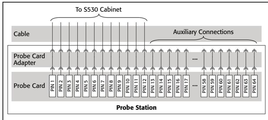
The Model 9139A PCA can be configured for auxiliary I/O connections, allowing instruments to be connected to it directly, bypassing the switch matrix signal paths. This provides for maximum bandwidth to the test structure with a minimum number of variables.
