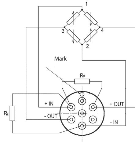
Fig. 3: Electrical connections Type RHU50...
