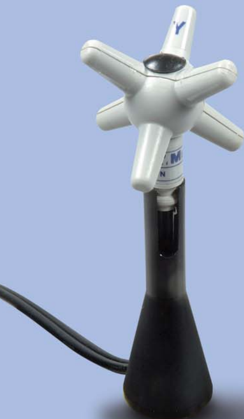
EP-600 mounted on tripod RF-transparent tip
