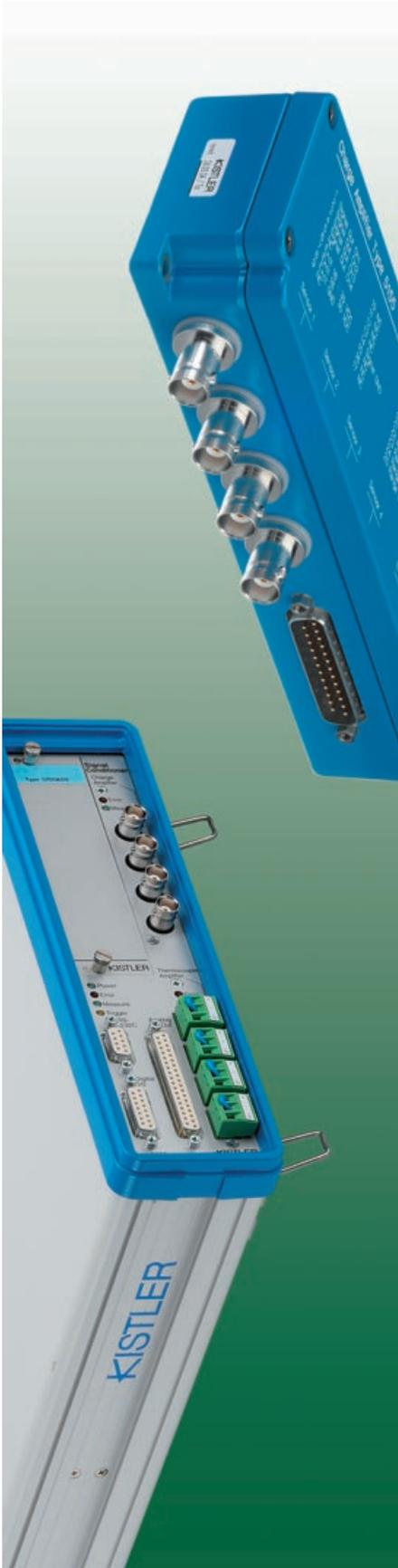
Charge amplifiers convert charges transmitted by a piezoelectric pressure sensor into a proportional voltage, which can be used as an input variable for monitoring and control processes. Kistler supplies a wide range of different charge amplifiers such as single-channel charge amplifiers or multi-channel amplifiers for charge and temperature.
