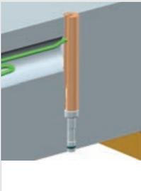
Accurate pressure data that is suitable for analysis can only be acquired by means of reliable and precise measuring technology. The mold cavity pressure can be measured directly, indirectly or in combination with the contact temperature. The position of the sensors within the mold plays a crucial role in this process.
