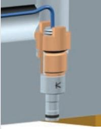
Sensor fitted into the drilled hole with sleeve
