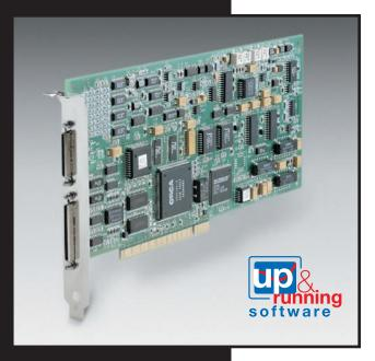
The KPCI-3116A is ideal for applications that require demanding measurements. It offers a great combination of high resolution, speed, high channel count, and quality that few other boards can match. Use the KPCI-3116A when you're developing a new product or interpreting physical phenomena.
