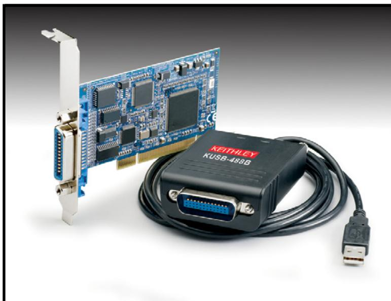
Keithley's GPIB interface solutions make it easy to add standard IEEE-488.2 bus control to any PC system. These high speed tools can control as many as 14 GPIB instruments or other devices over a distance of up to 20 meters. They are ideal for use with automated test equipment in laboratory and industrial applications.
