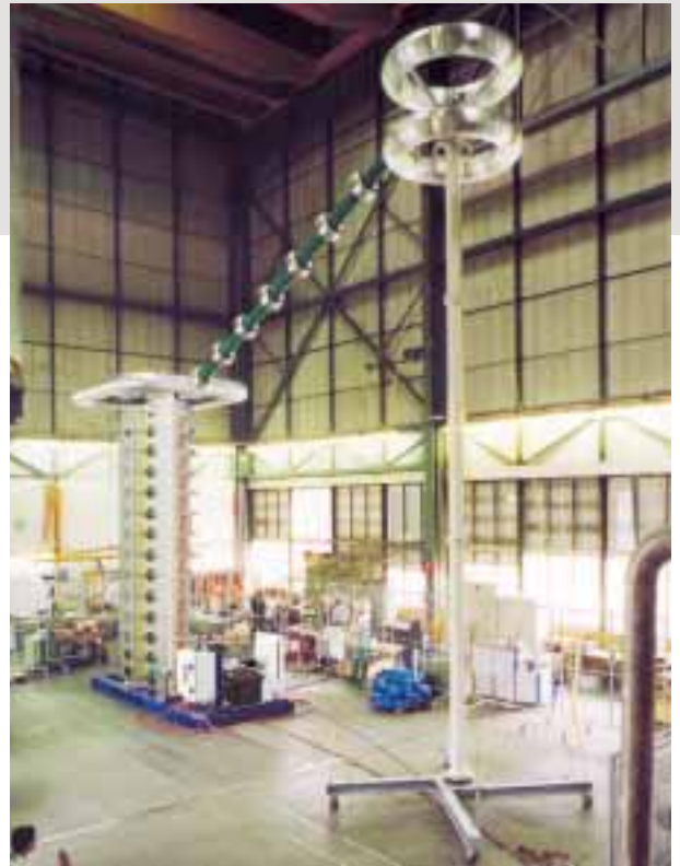
Impulse test system SGΔ A-L 1400-70 for oscillating switching impulse
