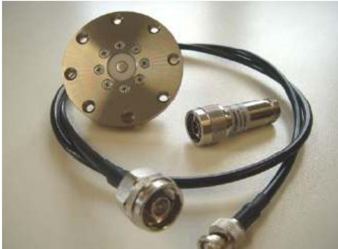
The Calibration Set has been developed as a tidy unit with the cable, attenuator and measuring target required to perform IEC/EN 61000-4-2 calibrations.
