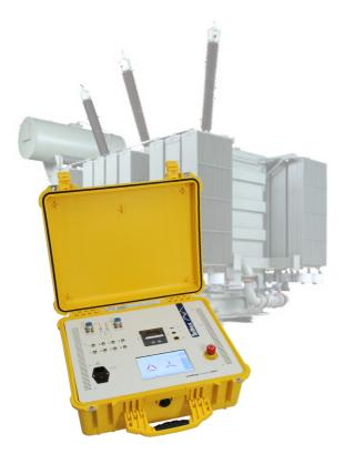
The Tettex 2293 is the result of extensive research and years of experience testing transformers. It incorporates a fast and highly advanced procedure to measure winding resistance. A simple one-time-connection system together with the simultaneous winding magnetization method drastically reduces measuring time.
