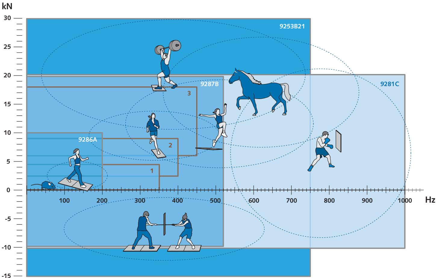
Kistler force plates are versatile and suitable – depending on maximum load capacity and natural frequency – for a wide variety of applications. In comparison three typical force plates with strain gage (4,5, 9 and 18 kN) and only limited application fields
