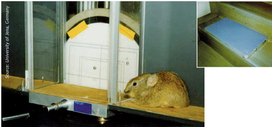
Special-sized force plates, e.g. for stairs (270x500x35 mm, top right) or for experiments with small animals (120x200x35 mm, top), are developed to customer requirements
