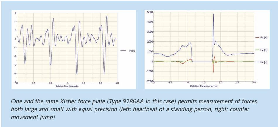
One and the same Kistler force plate (Type 9286AA in this case) permits measurement of forces both large and small with equal precision (left: heartbeat of a standing person, right: counter movement jump)
