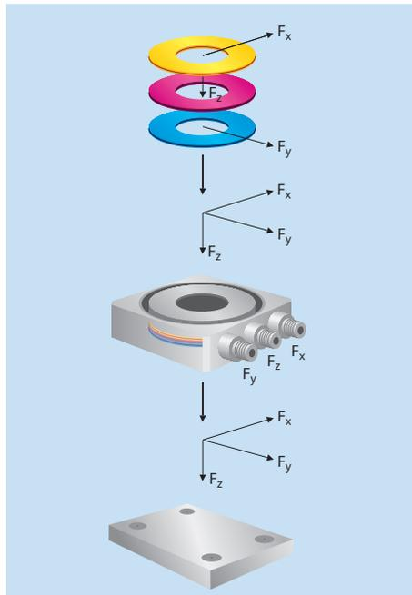
Principle of operation of multicomponent force plate
