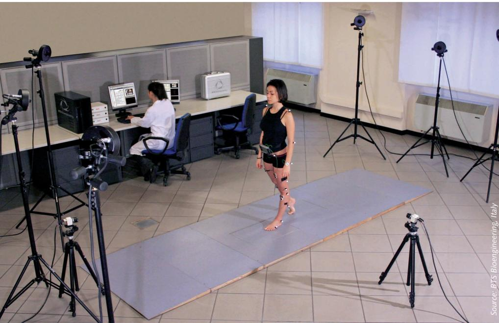
Gait analysis laboratory with infrared cameras and force plates Type 9286AA
