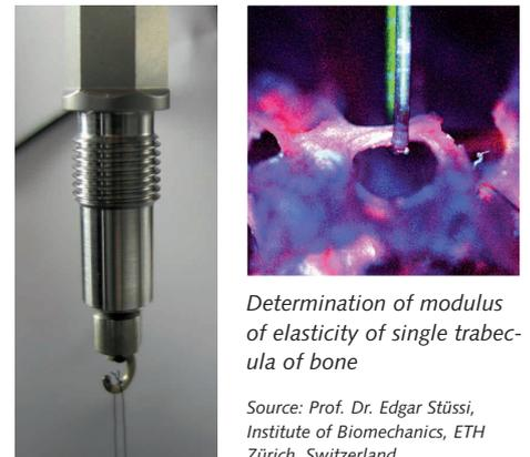
Determination of modulus of elasticity of single trabecula of bone
