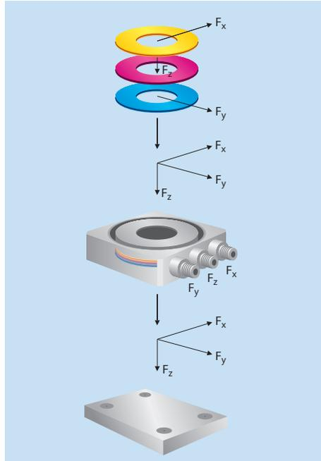
Principle of operation of multicomponent force plate
