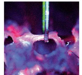
Determination of modulus of elasticity of single trabecula of bone
