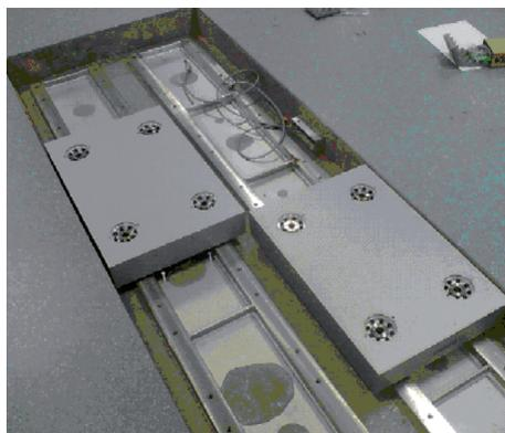
Easy installation and versatility: Two force plates Type 9281CA on frame with variable mounting positions
