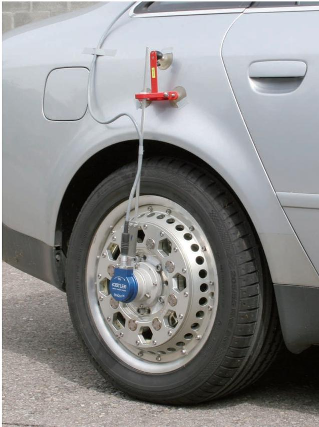
Fig. 1: Torque measuring wheel RoaDyn® P106 PremiumLine with slip ring module PremiumLine Type 9873
