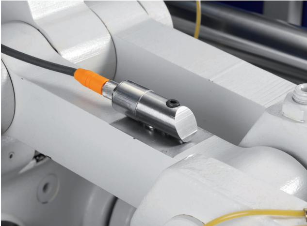
Fig. 8: Indirect force measurement on knuckle joint
