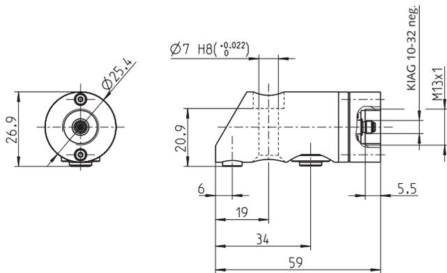
Fig. 2: Type 9237A20 with M13x1 adapter for protective hose
