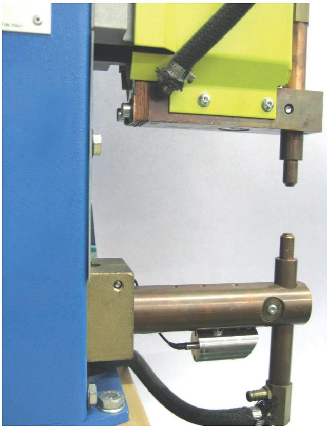
Fig. 6: Indirect measurement of electrode clamping force on a spot welding machine with strain sensor Type 9237A10
