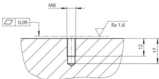
Fig. 3: Preparing the mounting surface
