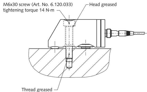
Fig. 5: Mounting with 6-point socket head cap screw
