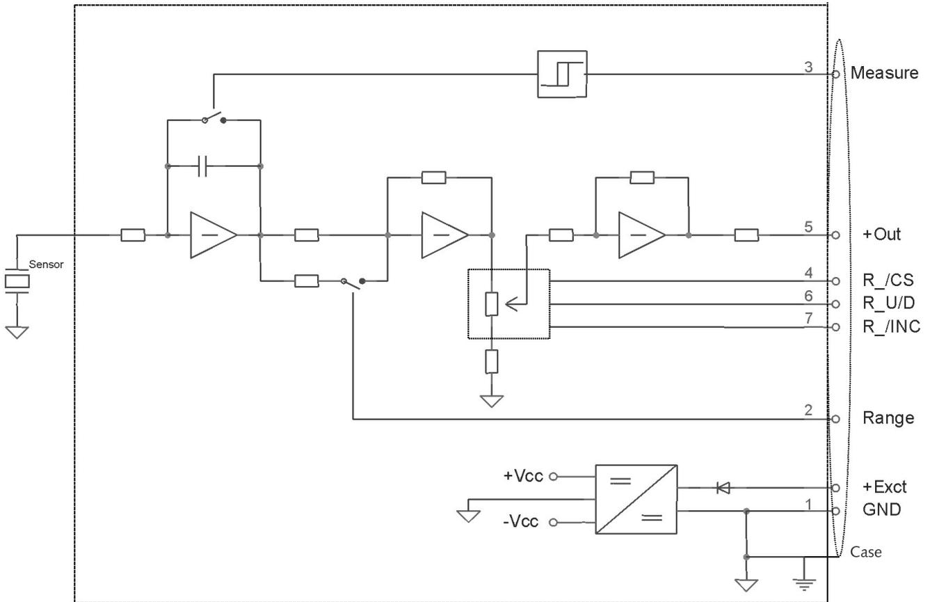
Fig. 10: Schematic diagram strain transmitter Type 9234A...
