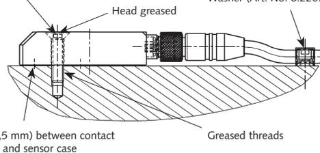
Fig. 4: Mounting by means of a countersunk screw
