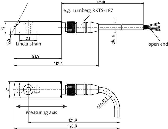
Fig. 8: Strain transmitter Type 9234Ax0
