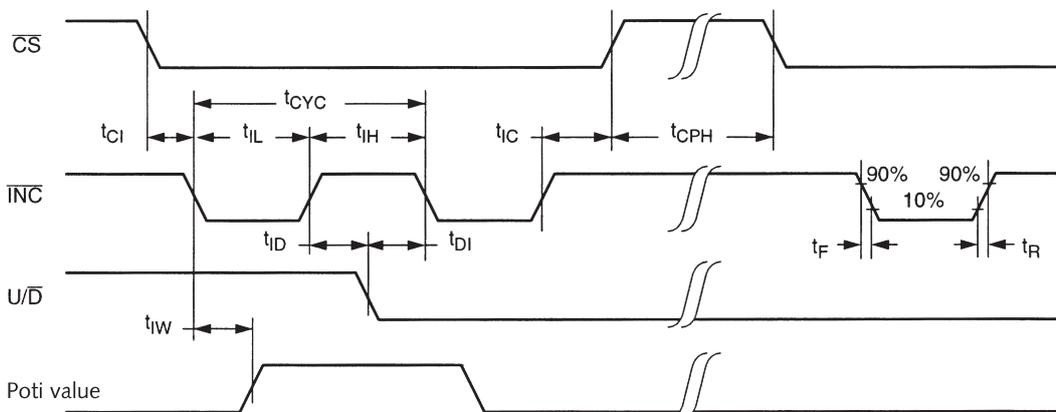
Fig. 11: AC control signals
