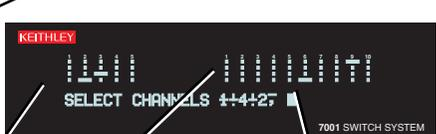
Multiplexer card display. The first row across represents channels 1 to 10. The second row is channels 11 to 20. Only the available channels are displayed.
