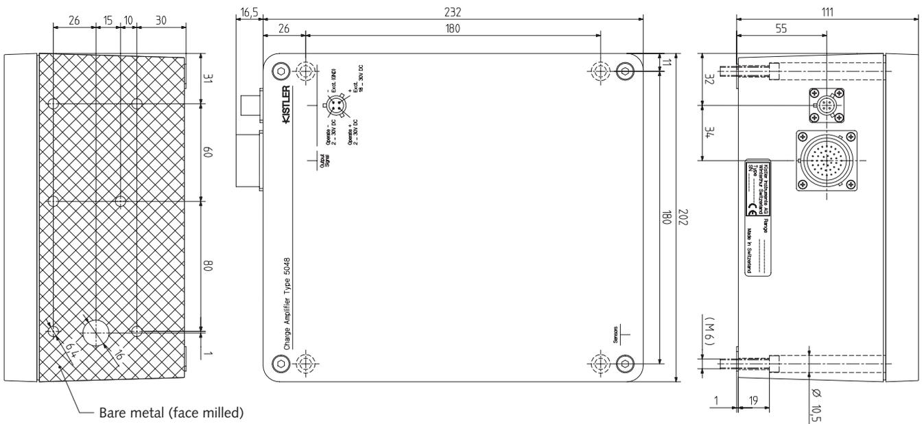
Fig. 2: Multi-channel charge amplifiers Type 5048A... (16, 24 or 32 channels)
