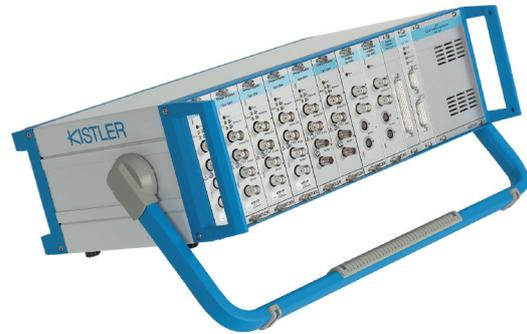
SCP for 8 Measuring Modules Type 2853A...
