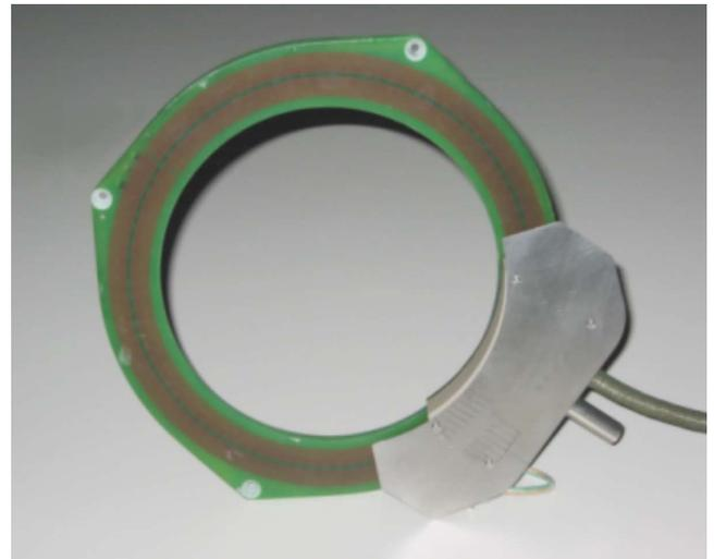
Fig. 1: In-board transmission consisting of rotor and stator
