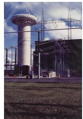
Impulse current testing arrangement for MV arresters
